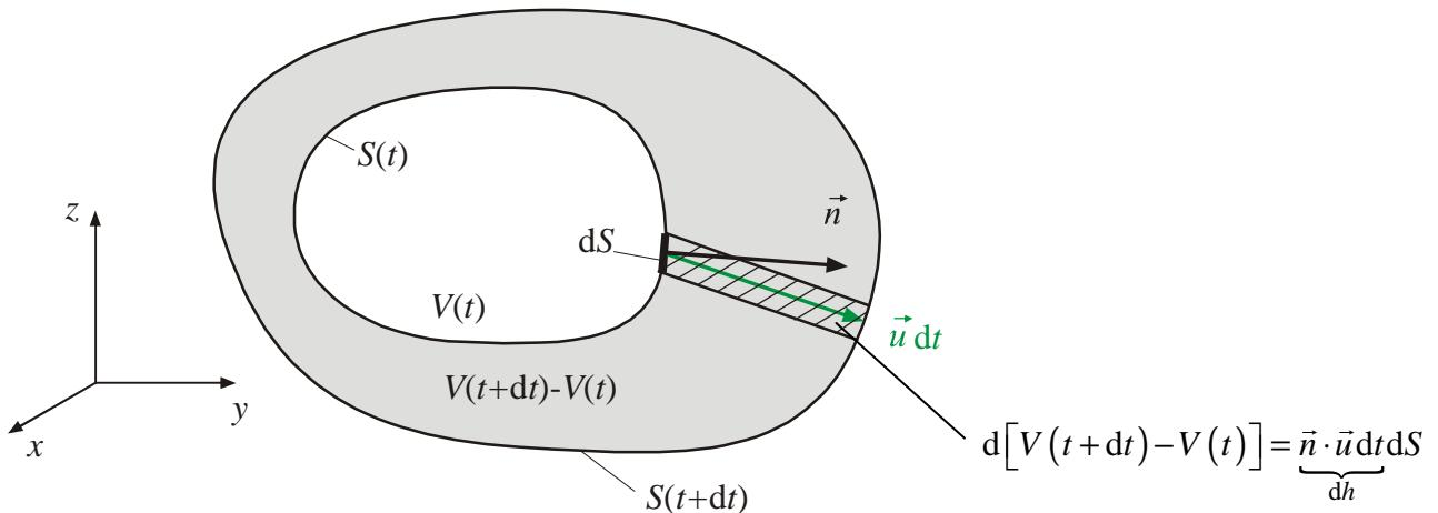
$$\frac{dV(t)}{dt} = \frac{V(t+dt) - V(t)}{dt} = \frac{\int_{S(t)} \vec{u} \cdot \vec{n} dS}{dt}$$
