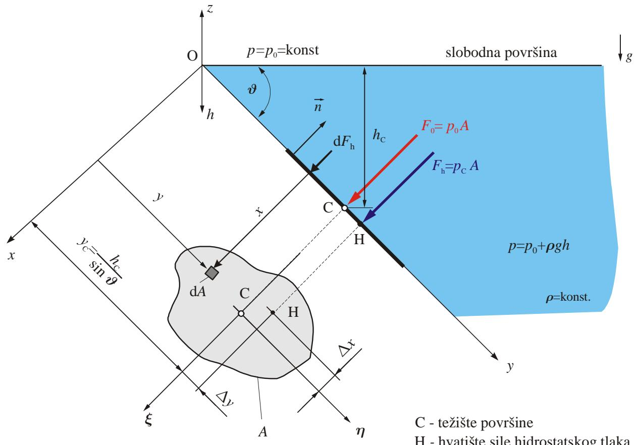
$$p = \underbrace{p_0}_{\text{konstantni tlak}} + \underbrace{\rho gh}_{\text{hidrostatski tlak}}$$
