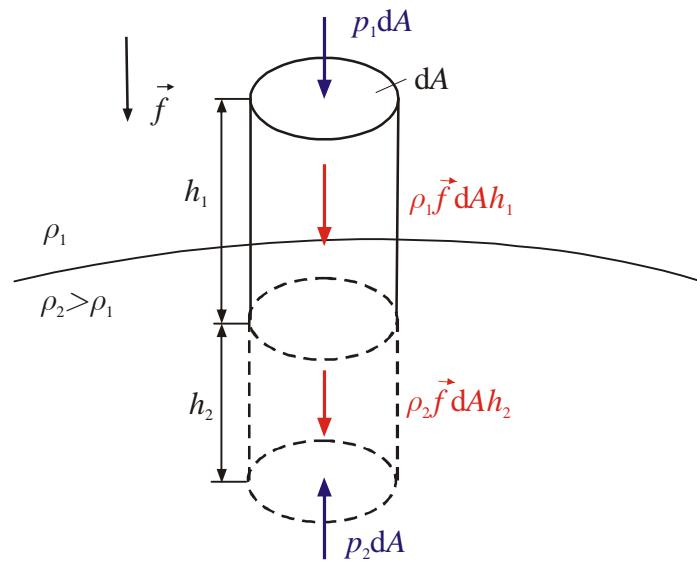
Ravnoteža sila:  $\lim_{\substack{h_1 \rightarrow 0 \\ h_2 \rightarrow 0}} [p_2 dA = p_1 dA + \rho_1 f dA h_1 + \rho_2 f dA h_2] = 0$
