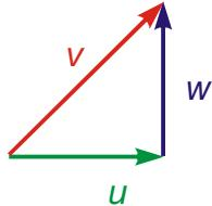
$$v_\vartheta = u_2 = \omega R$$
