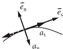
$$\vec{a} = \underbrace{v \frac{dv}{ds}}_{\text{tangencijalna komponenta ubrzanja}} \vec{e}_s - \underbrace{\frac{v^2}{R}}_{\text{normalna komponenta ubrzanja}} \vec{e}_n = a_t \vec{e}_s + a_n \vec{e}_n$$
