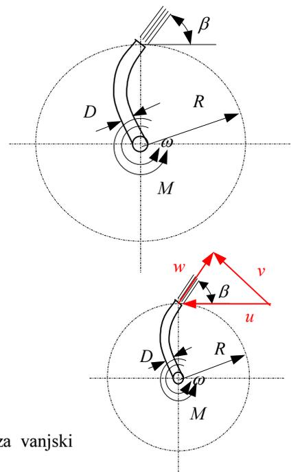
$$u = w \cdot \cos(\beta) \quad \omega = \frac{u}{R} \quad \omega = 18.378 \text{ s}^{-1} \quad N = \frac{\omega \cdot 30}{\pi}$$
