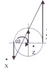
$$\dot{\omega} = \frac{\dot{x}}{p} = \frac{\dot{y}}{2R-p} = \frac{\dot{x} + \dot{y}}{2R} = \frac{\dot{y} - \dot{x}}{2(R-p)} = \frac{\dot{z}}{R-p}$$
