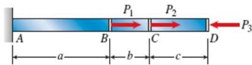
$$\begin{array}{lll} E := 200 \text{ GPa} & a := 1.5 \text{ m} & P_1 := 12 \text{ kN} \\ A := 0.4 \text{ cm}^2 & b := 0.5 \text{ m} & P_2 := 8 \text{ kN} \\ & c := 0.75 \text{ m} & P_3 := 6 \text{ kN} \end{array}$$
