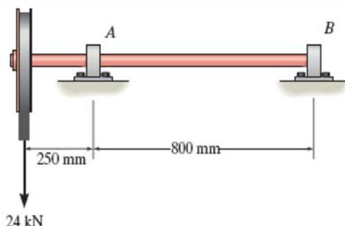
$$\begin{array}{lll} F_{\text{m}} := 24 \text{kN} & L_1 := 0.25 \text{m} & \sigma_{\text{doz}} := 150 \text{MPa} \\ & L_2 := 0.8 \text{m} & \tau_{\text{doz}} := 100 \text{MPa} \end{array}$$
