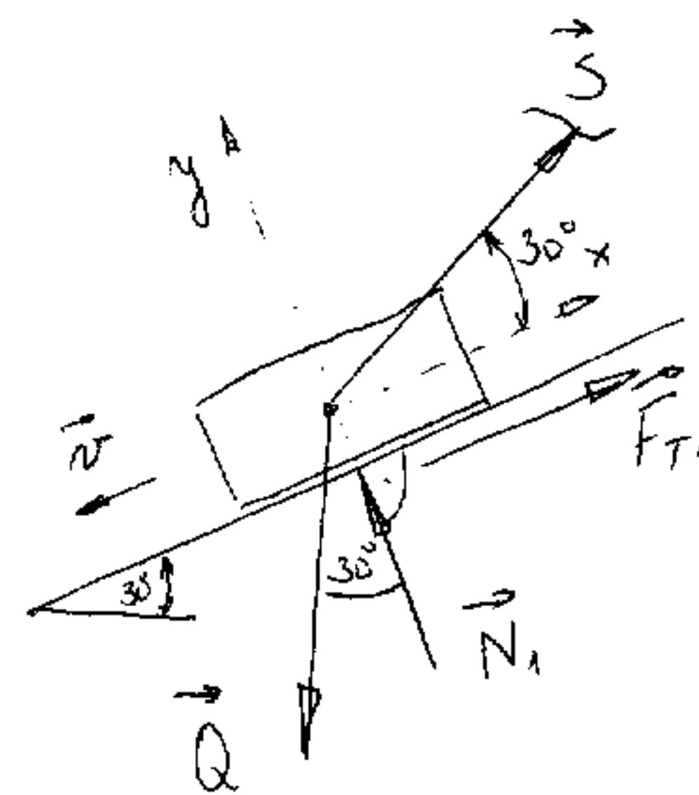
$$\sum X = 0 \quad S \cos 30^\circ + F_{T_1} - Q \sin 30^\circ = 0 \quad \dots (1)$$
