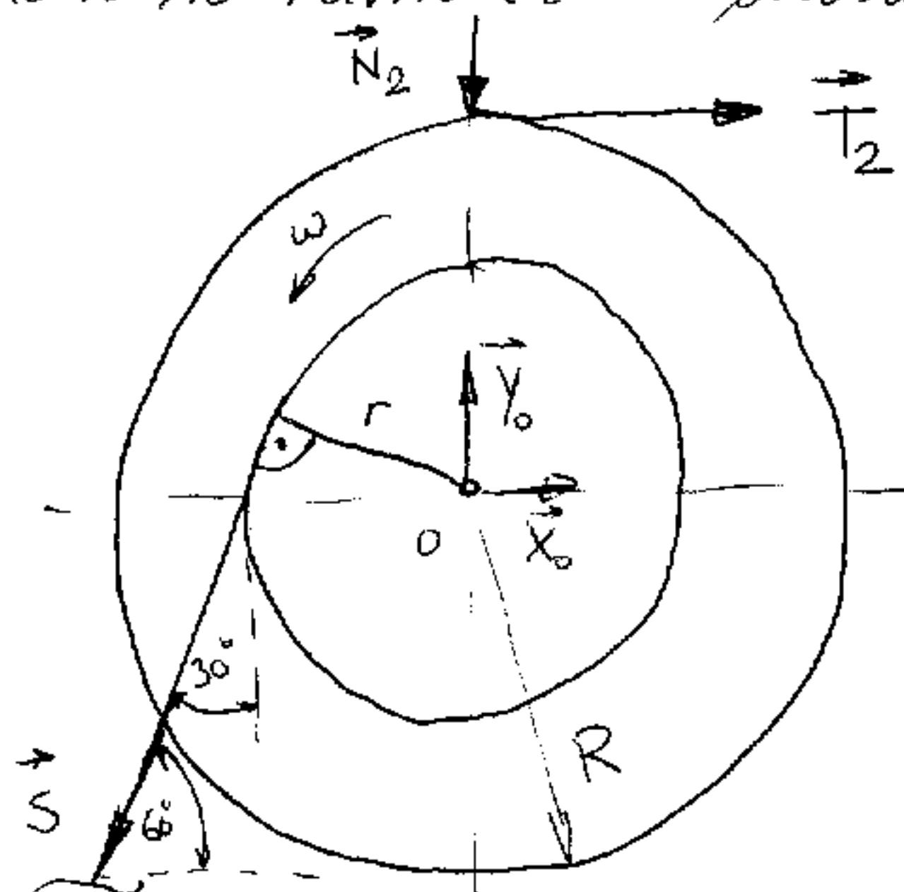
$$\sum X = 0 \quad X_0 + T_2 - S \sin 30^\circ = 0 \quad \dots (1)$$
